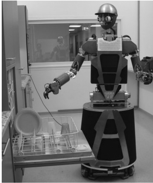
Fig. 4.1 The humanoid robot ARMAR-III. The has 43 DOF. From the kinematics control point of view, the robot consists of seven subsystems: head, left arm, right arm, left hand, right hand, torso, and a mobile platform.
