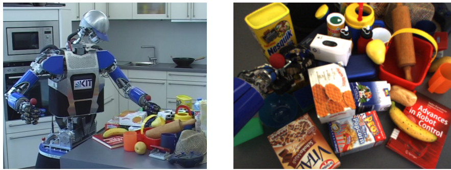
Fig. 13: ARMAR-III pushing an object in a cluttered scene to segment it.
