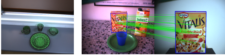
Fig. 7: Object recognition of daily objects based on shape information and appearance features.
