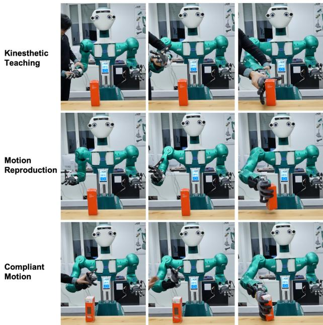
Figure 7. Kinesthetic teaching and compliant motion reproduction based on task space impedance control. During motion execution, the robot is able to compliantly adapt its action to external force perturbations and to safely interact with humans.
