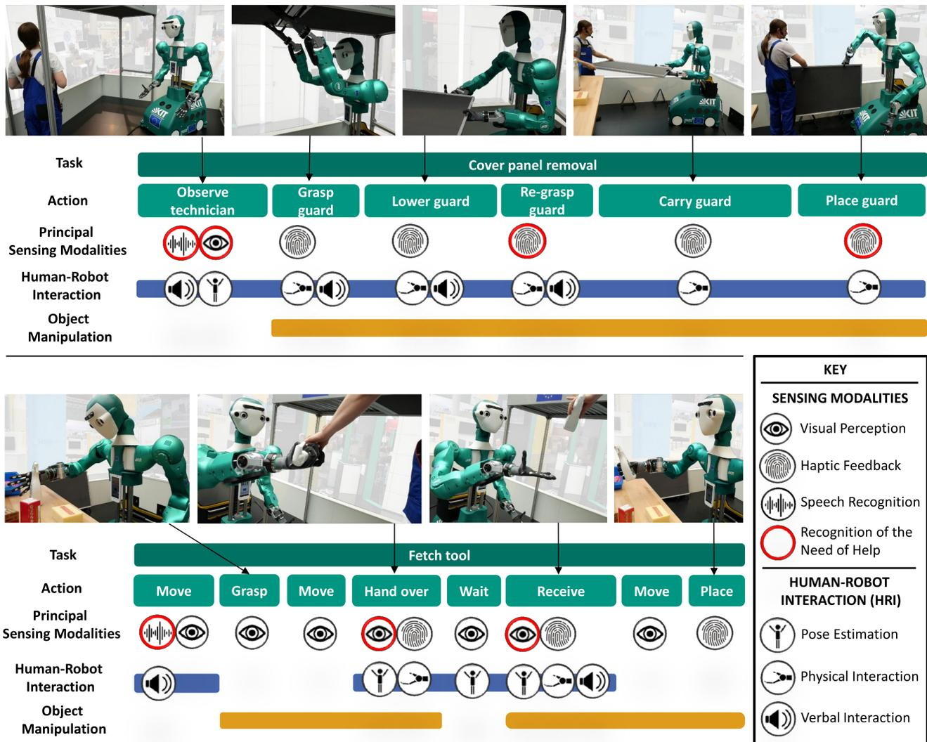
Figure 10. The warehouse demonstration scenario broken down into tasks, actions, principal sensor modalities, human-robot interaction modalities and object manipulation. On the top, the compliant collaborative manipulation is shown in a *cover panel removal* task. On the bottom, autonomous mobile manipulation is demonstrated with *fetching a tool* for the technician.
