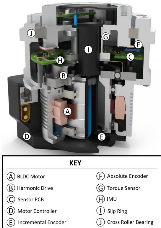
Figure 3. Rendered 3D cross-section of the mid-sized sensor-actuator-controller (SAC) unit. The dual arm system of ARMAR-6 has 16 highly integrated SAC units in three different sizes.
