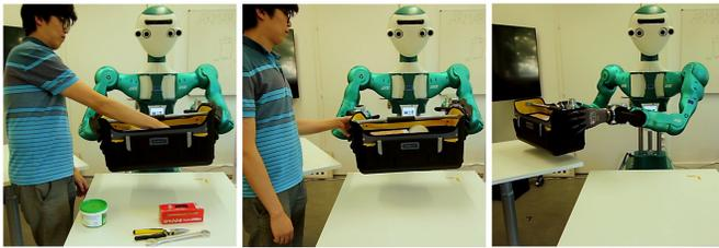
Figure 8. The compliant bimanual control system allows manipulating large and heavy objects. **Left:** Holding a toolbox filled with objects with a total weight of 6kg. **Middle:** The coupling of both arms is guaranteed by the bimanual controller during perturbations. **Right:** The motion is encoded with CC-DMP and the forces exerted on the toolbox are generated by the bimanual controller.
