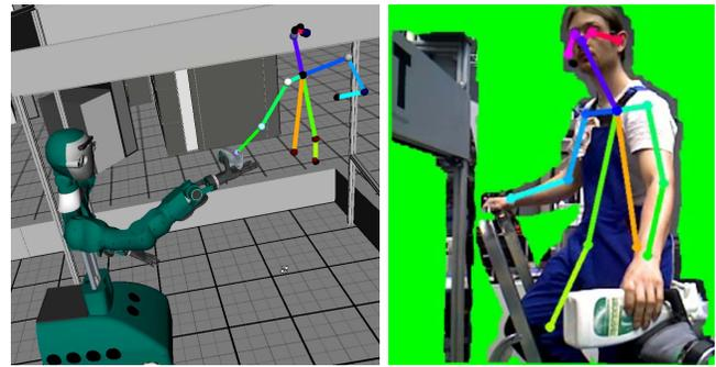
Figure 9. Active handover of a tool between ARMAR-6 and the human technician. The robot uses marker-free 3D human pose estimation and force feedback to recognize the human’s intentions to provide help when needed.
