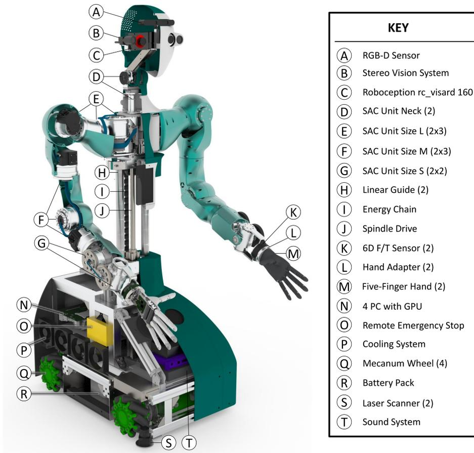
Figure 2. Visualization of essential internal components (A-T) of ARMAR-6.
