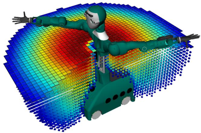
Figure 4. Sectional view through the  $10.7 \text{ m}^3$ , nearly ellipsoidal workspace of the dual arm system incorporating the prismatic joint of the torso. The color of the voxels correspond to the local manipulability as described by Yoshikawa [22] with the extension that the manipulability maps for both arms are merged into one manipulability map. The warmer the color, the higher the manipulability.
