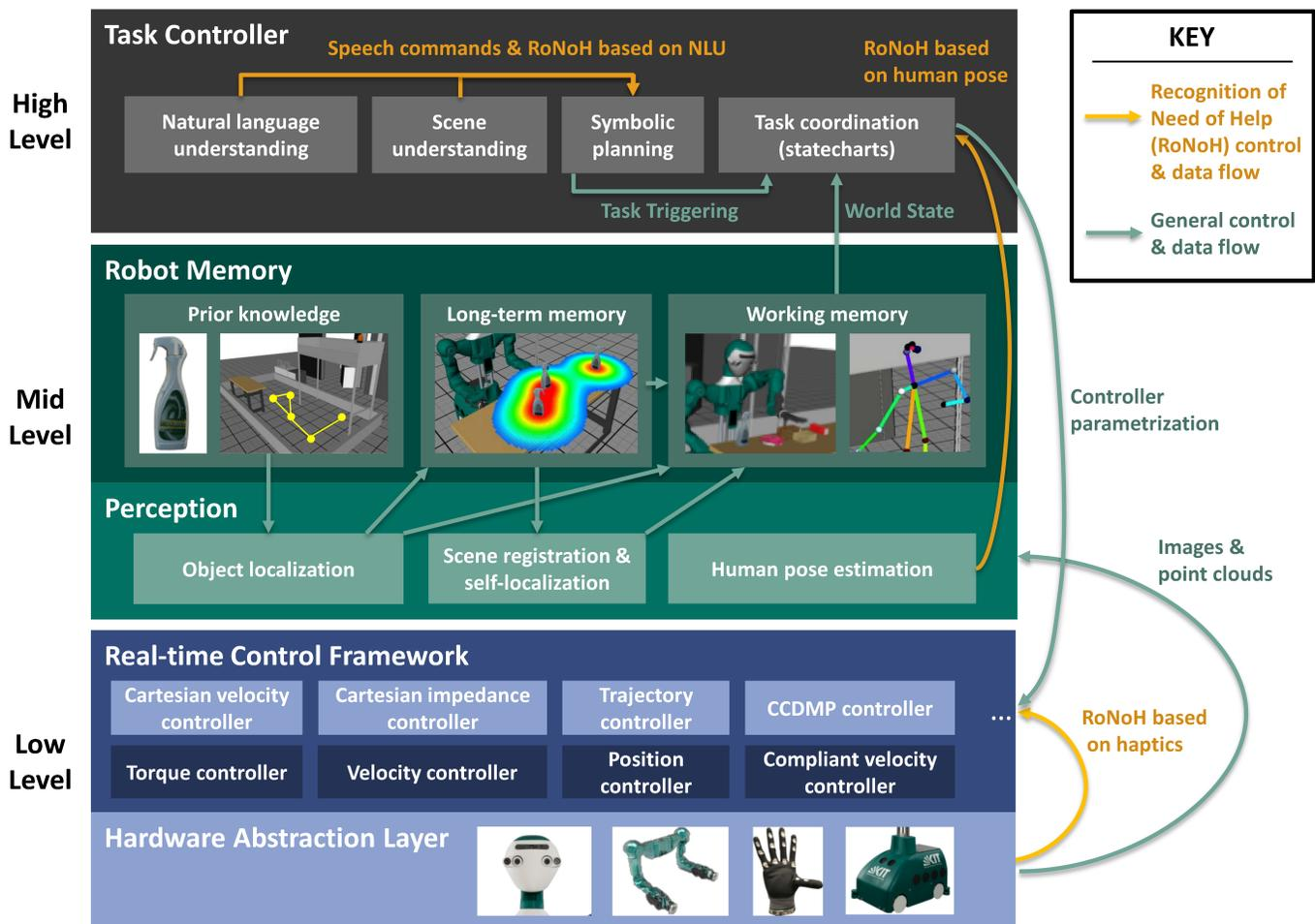
Figure 5. Overview of ArmarX as the functional software architecture of ARMAR-6. The depiction is divided into its three main conceptual levels and their principal interconnections. The information is increasingly abstracted from the low level (e. g. raw sensor values) to the high level (e. g. symbolic predicates).
