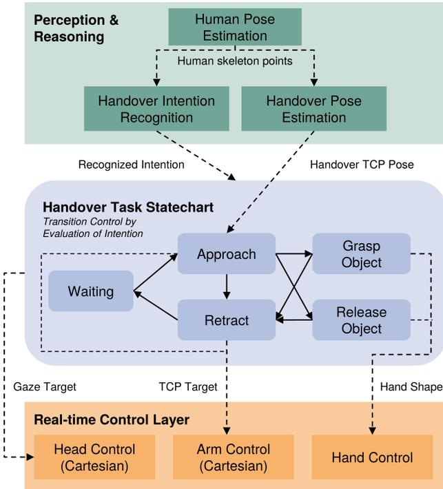
Figure 6. Flowchart of the handover task showing the coordinating statechart as well as the involved perception and control modules needed for an interactive and adaptive handover.
