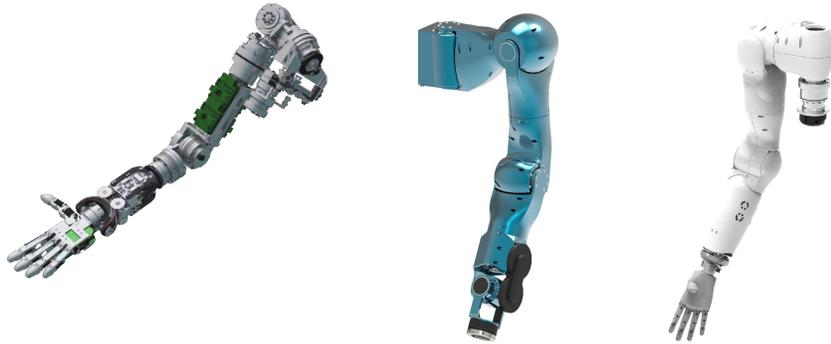
Fig. 9: Arm designs of humanoid robots: In contrast to the arm of ARMAR-4 [4] (left) that uses a frame construction, the arms of ARMAR-6 (middle) and ARMAR-7 (right) use an exoskeleton design.
