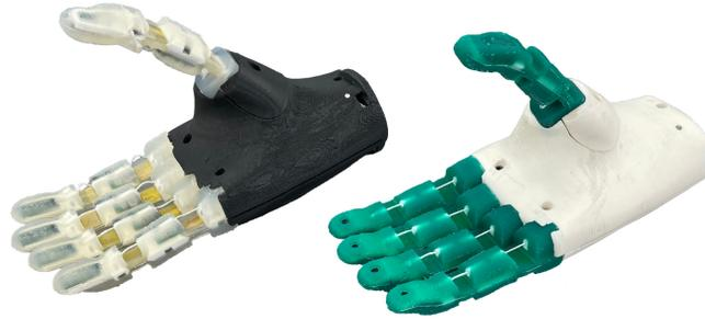
Fig. 13: The *KIT Sensorized Soft Hand* and *KIT Finger-Vision Soft Hand* [55]
