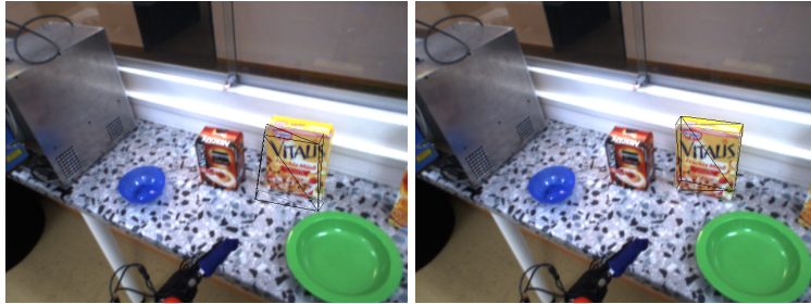
Fig. 3. Result of 6-DoF pose estimation. Left: using the conventional monocular approach. Right: using the proposed stereo-based approach.
