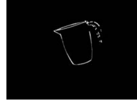
Fig. 6. Result of the bitwise AND operation (before summation) for the right images from the Figs. 4 and 5. As can be seen, the similarity of the particle pose and the real pose lead to a relatively large overlap.
