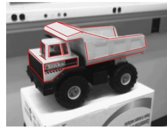
Fig. 2. Typical 3D model for model-based tracking composed of straight line segments, as used in [8].
