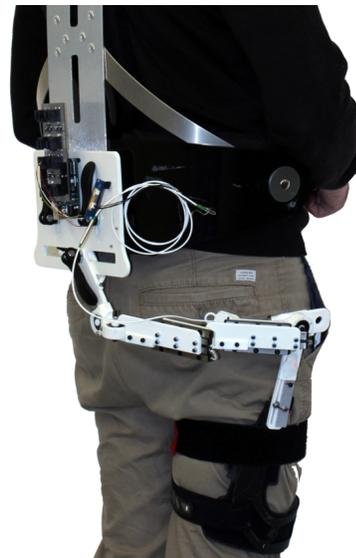
Fig. 1. 3D printed prototype of the proposed hip joint of a lower limb exoskeleton
