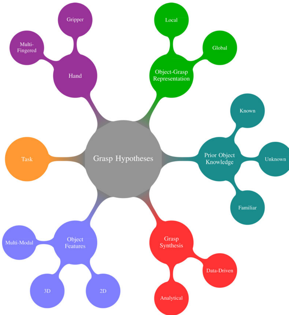
Fig. 1. We identified a number of aspects that influence how the final set of grasp hypotheses is generated for an object. The most important one is the assumed prior object knowledge , as discussed in Section I-D. Numerous different object-grasp representations are proposed in the literature that are relying on features of different modalities such as 2-D or 3-D vision or tactile sensors. Either local object parts or the object as a whole are linked to specific grasp configurations. Grasp synthesis can either be analytic or data-driven. The latter is further detailed in Fig. 2. Very few approaches explicitly address the task or hand kinematics of the robot.
