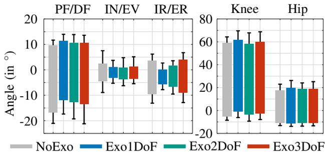
Fig. 8: RoM depiction for all three ankle rotations, knee and hip joint during straight walking for all configurations (*NoExo*, *Exo1DoF*, *Exo2DoF* and *Exo3DoF*). The blocks represent the maximum and the minimum angle of Fig. 6. The standard deviation (vertical error lines) values shows variability between the participants.
