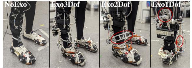
Fig. 3: A participant without and with the ankle exoskeleton in its three configurations. The parts added to fix certain DoF are marked in red.
