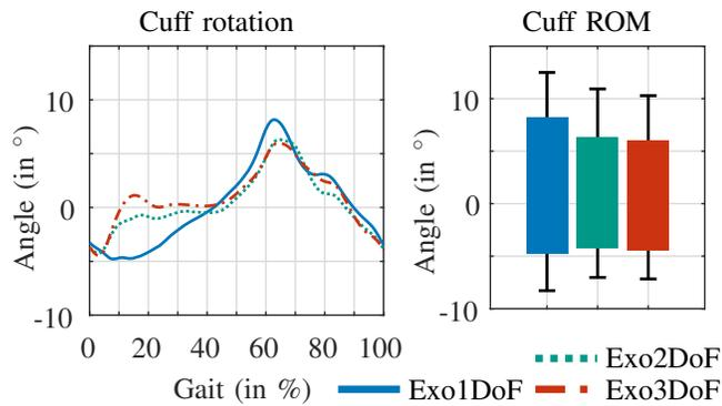
Fig. 10: Illustration of the cuff rotation and RoM. This is the rotation of the cuff relative to the knee on the axis of the shank. (left) The average cuff rotation for all strides of all participants shown for each condition, (right) the RoM depicted as a bar chart where the error ticks represent the standard deviation of all strides capturing the variability between participants.
