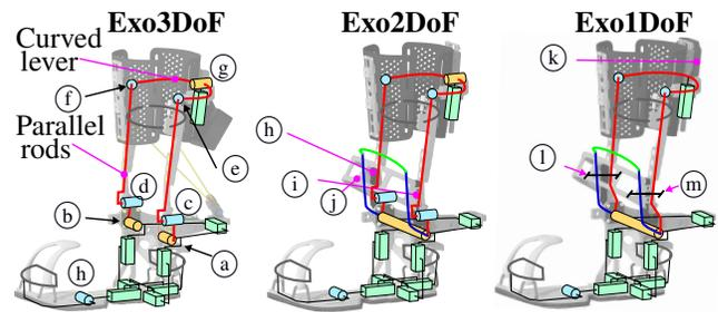
Fig. 2: Illustration of the three exoskeleton configurations: *Exo3DoF*, *Exo2DoF*, and *Exo1DoF*. The kinematic structure comprises various joint types: a hinge joint represented by "blue cylinder", a ball joint "blue sphere", a hinge joint with angle measurement "yellow cylinder", and an adjustable translation joint "green rectangle". The explanations for each callout are provided in the text. (adapted from [8])
