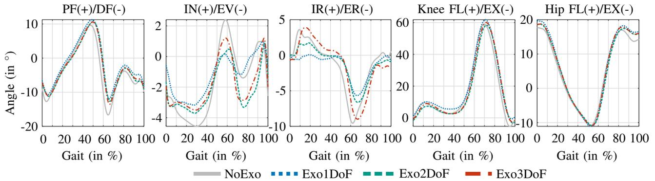
Fig. 6: Illustration of the user’s kinematics: ankle plantar-/dorsiflexion (PF/DF), in-/eversion (IN/EV), internal/external rotation (IR/ER), knee flexion/extension (FL/EX) and hip flexion/extension (FL/EX). The plots depict the average of all strides for each configuration, highlighting the differences in kinematics between the four exoskeleton configurations. The motion direction is indicated in the title of the subfigures.
