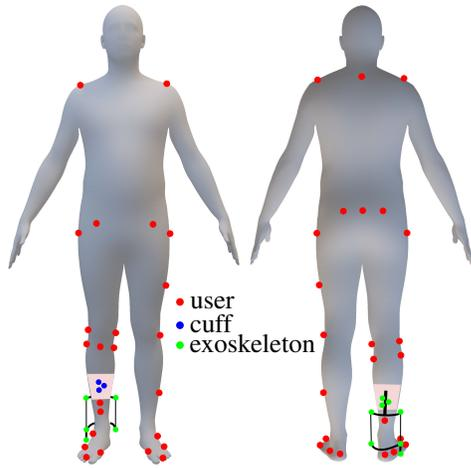
Fig. 4: Illustration of the MOCAP marker positions on the exoskeleton and the user. Red markers are attached on the user. Blue markers are attached on the exoskeleton cuff. Green markers are attached on the exoskeleton.
