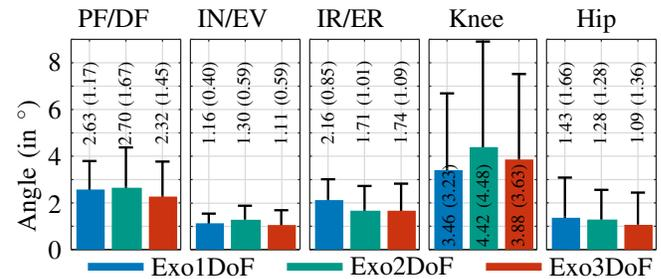
Fig. 7: Ankle rotation similarity of *ExoXDoF* to *NoExo* condition. The RMSE values are calculated between the averages of the respective configuration and the *NoExo* average for all strides of all participants. The standard deviation (vertical error lines) of RMSE values shows variability between the participants.
