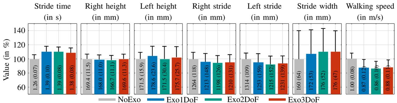
Fig. 9: Gait parameters normalized as percentage compared to the baseline for each condition. The gait parameters are the time of each stride (Stride time), average maximum foot height for either left or right leg (Right/Left height), length of the stride (Right/Left stride) and width of the stride (Stride width). The actual value and standard deviation are written in the respective column. The vertical error lines represent the standard deviation, indicating the variation between participants.
