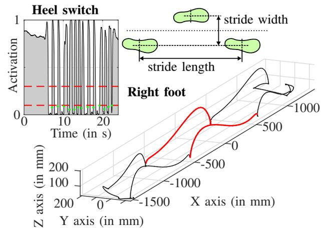
Fig. 5: Illustration of several relevant parameters relevant for this paper: (top left) heel switch activation example and detected strides in green, (top right) definition of the stride length and width, (bottom) an example of two segmented strides of the left leg.
