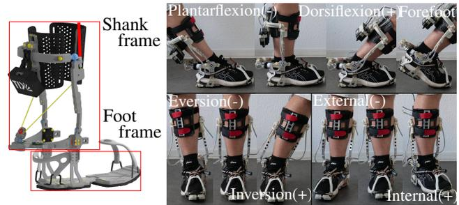
Fig. 1: Illustration of exoskeleton components and movements. (left) The shank and foot sections of the exoskeleton. (right) Demonstration of the exoskeleton's functionality, showcasing the three primary ankle joint rotations: plantar-/dorsiflexion (PF/DF), in-/eversion (IN/EV), and internal/external rotation (IR/ER), along with the forefoot rotation of the foot frame. (adapted from [8])
