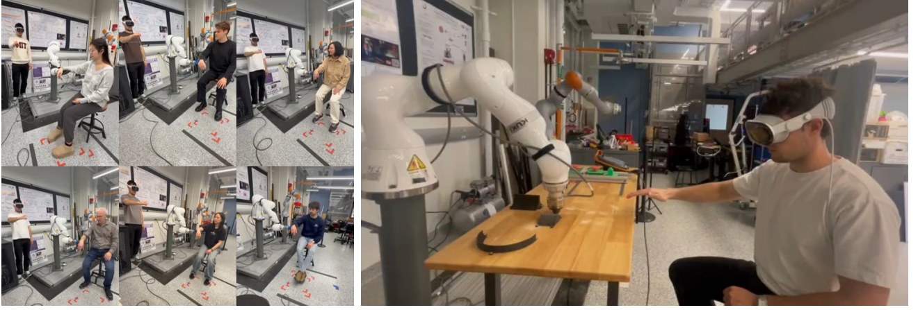
Fig. 6: Examples of teleoperated demonstrations used for training. (Left) Physical therapy dataset with robotic-assisted upper-limb tasks. (Right) Parkour dataset with free-space and contact-rich motions across obstacles.
