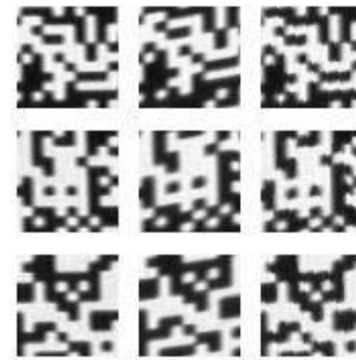
Fig. 2. Three local sample patterns for demonstration of the Gruen Algorithm; each left pattern in a row is a template pattern, each middle one is the actually captured pattern (distorted by scene geometry) and each right one is the pattern after application of the Gruen Algorithm.
