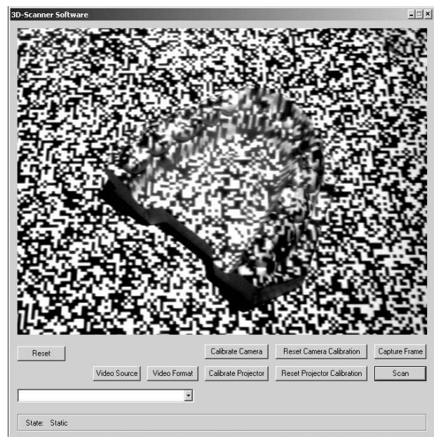
Fig. 4. Plaster Cast with projected Speckle Pattern
