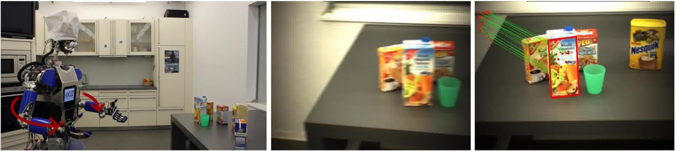
Fig. 6: Setup for the object localization experiment (left). The torso of the humanoid robot ARMAR-III is subjected to a sinusoidal perturbation while the objects are constantly localized. The image of the left foveal camera is shown for both the unstabilized case (center) and the stabilized case (right). In addition, the successful object localization result is visible in the stabilized case.
