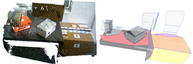
Fig. 3: Left : An exemplary point cloud of a cluttered tabletop scene. Right : Extracted geometric primitives. Higher semantic structures, e.g. boxes, are visualized with a gray volume.
