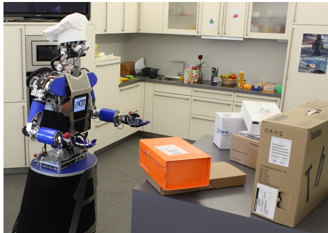
Fig. 1: The humanoid robot ARMAR-III performing a bimanual whole-body grasp to lift a box. The scene representation is iteratively fused from consecutive RGB-D images. Furthermore, our reasoning process allows for identification of higher semantic structures, i.e. structures composed of several geometric primitives. This allows to automatically extract and associate more complex actions, e.g. a bimanual lift, with the geometric primitives.
