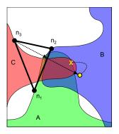
Fig. 4. Determining the next guess from a cycle consisting of the nodes  $n_1$ ,  $n_2$  and  $n_3$ . Node  $n_3$  is the worst node according to the sum of the displacement lengths to the constraints A, B and C. To determine the next guess configuration, the worst node  $n_3$  is reflected through the weighted average of the cycle's other nodes  $n_1$  and  $n_2$ . Projecting the guess configuration to constraint A then solves the problem.
