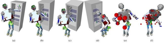
Fig. 6. Example configurations found by Constellation for each type of test scene. (a)-(d) Reaching tasks for shelves 1-4, respectively. (e) Randomlygenerated scene with 7cm spheres (f) Randomly-generated scene with 2cm spheres.
