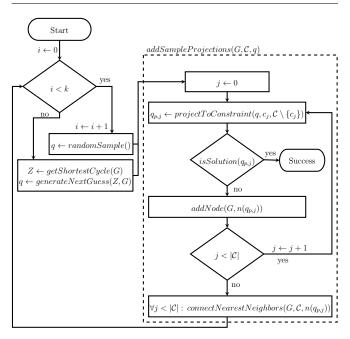
Fig. 2. Flowchart of the Constellation algorithm.
