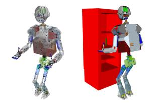
Fig. 5. Left: The set of collision points. Right: Voxelized refrigerator.
