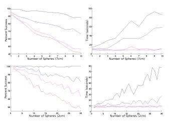
Fig. 7. Percent success and average runtime for solvable scenes of the sphere tests. Runtime averages were computed over successful runs of each algorithm. Black: Constellation, Blue: Cyclic-ns, Magenta: Cyclic, Red: Direct projection.
