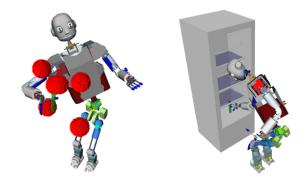
Fig. 1. The humanoid ARMAR-III [3], virtually enhanced with two 6 DOF legs (33 DOF total), reaching in cluttered environments while satisfying multiple constraints. The legs are a scaled-up version of the iCub legs [4].
