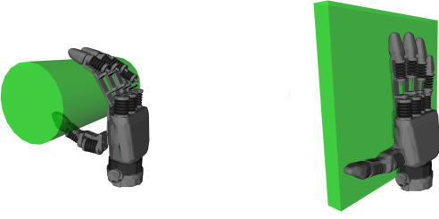
Fig. 3: The two grasp types considered throughout this work: a prismatic grasp (left) and a platform grasp (right).
