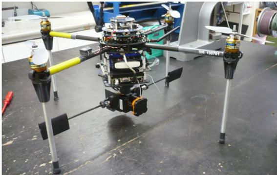
**Figure 5.** The prototype of the sensor assembly and other hardware necessary for data acquisition mounted under the payload section of a modified Skybit Systems Eagle quadcopter system.
