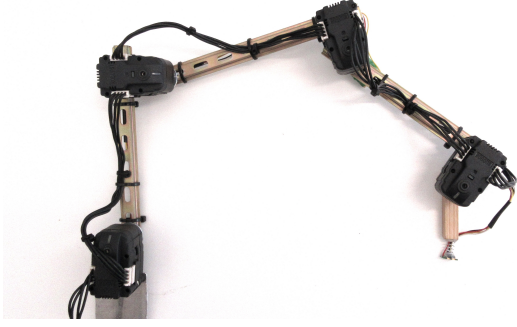
Fig. 3: The planar 4-DOF robotic arm that we use as test bed. The proposed surface orientation sensor is attached to the tip of the last link with a coil spring.
