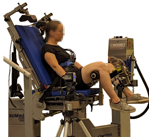
Fig. 1: The setup for isokinetic knee joint motion with a subject on the used IsoMed 2000 device.
