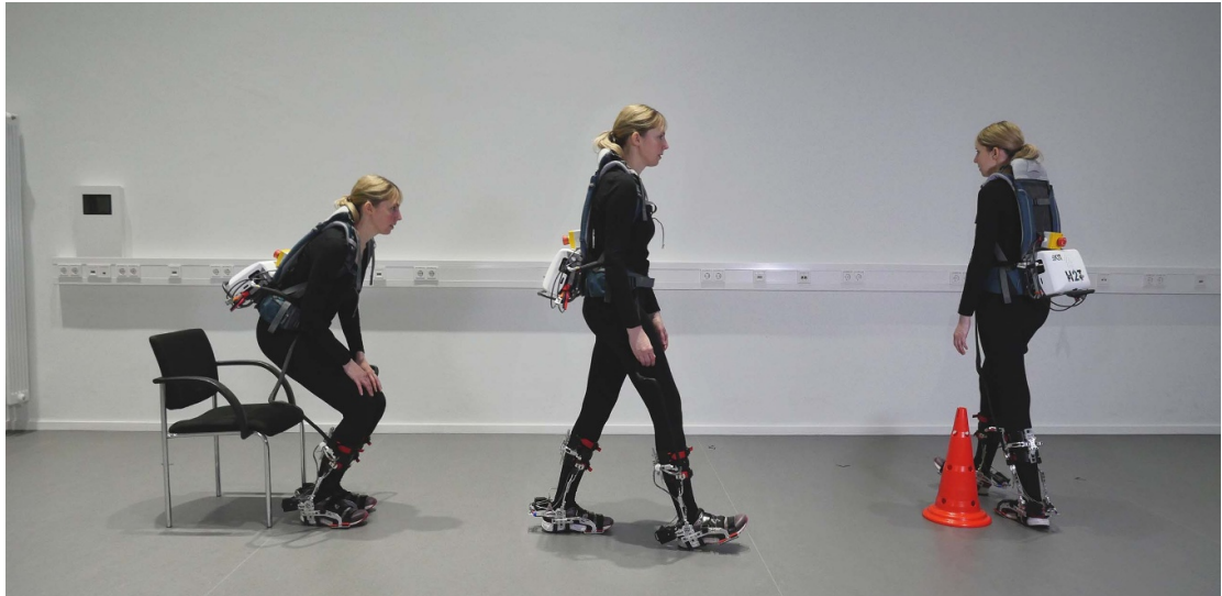
Figure 3. Exemplary realisation of a TUG test using a mobile ankle exoskeleton and its built-in sensors.
