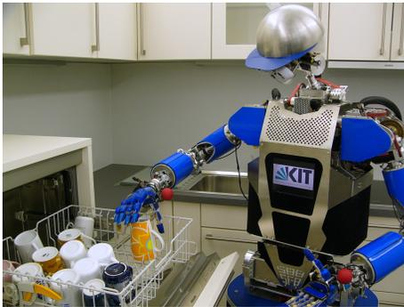
Fig. 13: The humanoid robot ARMAR-III [23] equipped with WEISS ROBOTICS tactile sensors [24] on the fingertips and in the palm.
