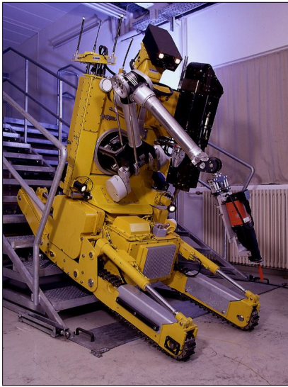
Fig. 7. KHG's robot capable of climbing stairs.
