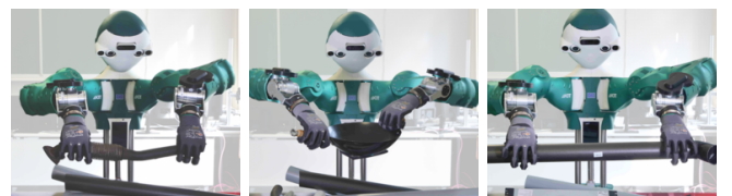
Fig. 7: The humanoid robot ARMAR-6 grasping and carrying multiple objects bimanually.
