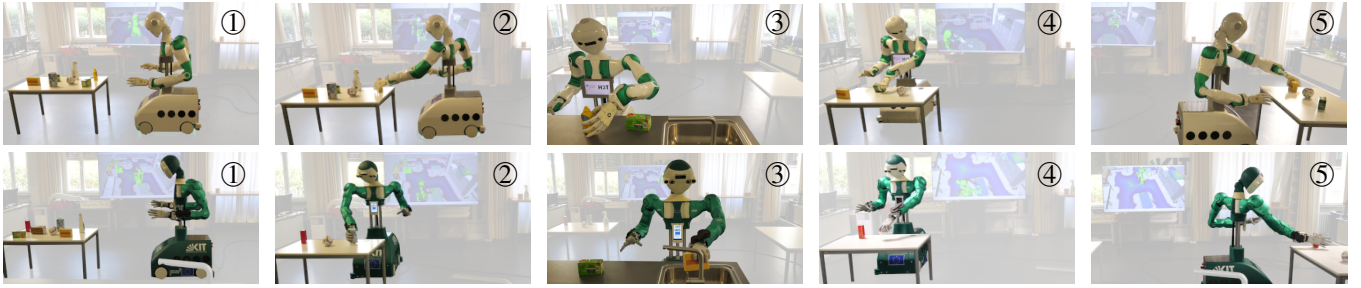
Fig. 8: Table-clearing of known and unknown objects with ARMAR-DE and ARMAR-6. ① Initial setup, ② grasping of known objects, ③ placing of known objects, ④ grasping of unknown objects, and ⑤ placing of unknown objects. An accompanying video shows the experiments.
