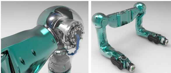
Fig. 9: SAC units in the KIT dual arm robot
