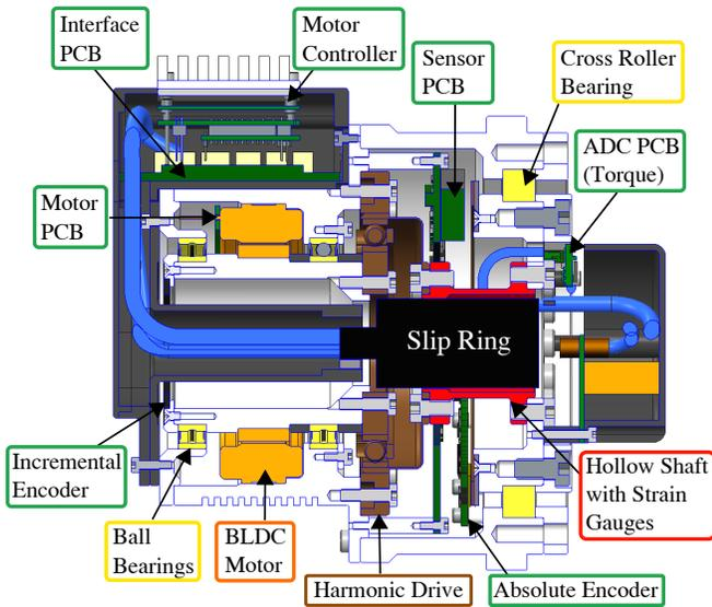
Fig. 2: Labeled cross section of the medium-sized SAC unit
