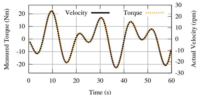
Fig. 7: Rotational velocity and measured torque during a velocity tracking experiment (scaled to match). The proportionality between the two values indicates correct functioning of the torque sensor
