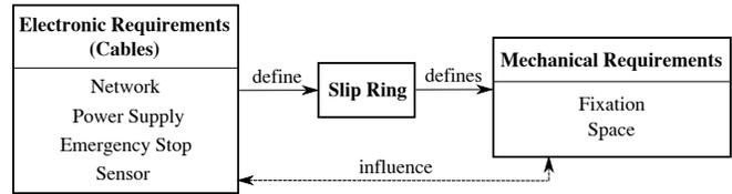
Fig. 3: Example of our electro-mechanical co-design: The slip ring has to fulfill electronic requirements and simultaneously it defines mechanical requirements
