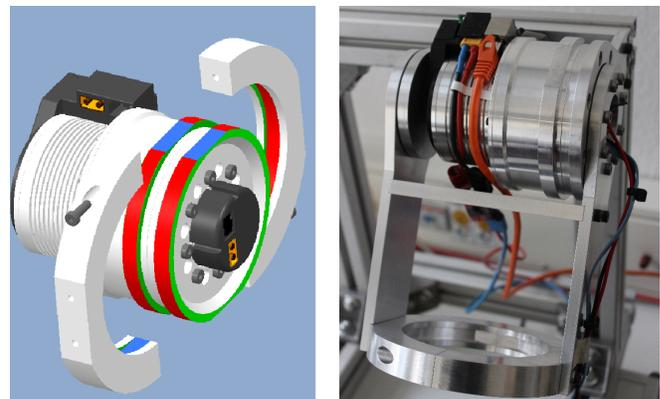
Fig. 5: Mechanical interfaces: Clamp ring interface highlighted in red (left); Flange interface used in an elbow joint (right)
