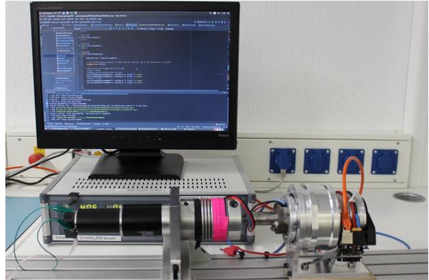
Fig. 6: Test rig for the SAC unit. The SAC unit on the right is connected to an electrodynamic brake on the left (black) by a bellows coupling
