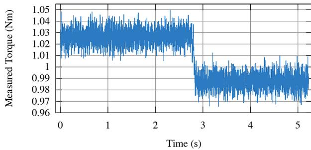
Fig. 8: Torque sensor response to a sudden change in the applied torque of 0.04 N m
