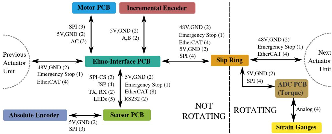
Fig. 4: Overview over the electrical connections between components in the SAC unit. Numbers in brackets indicate the number of wires needed for the particular connection
