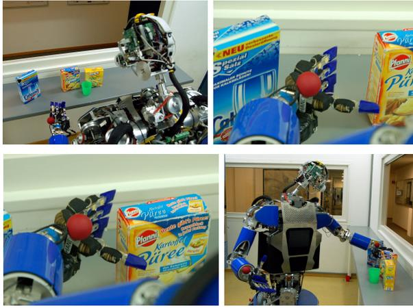
Fig. 10. ARMAR-III is executing a planned trajectory by the proposed visual servoing techniques.
