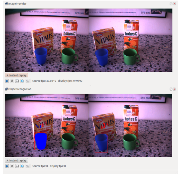
Figure 8: The VisionX image provider stream (top) and the corresponding output of an image processor related to single colored object recognition (bottom).
