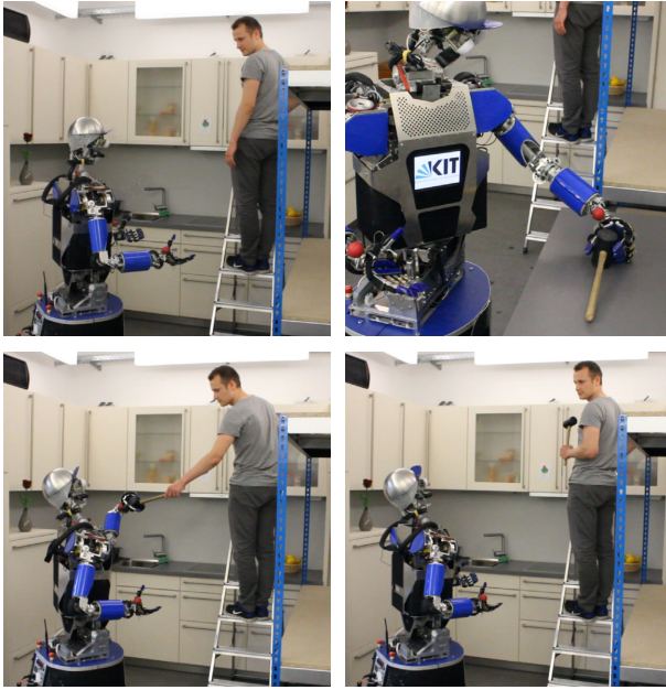
Fig. 8. A hand over task executed with ARMAR-III.
