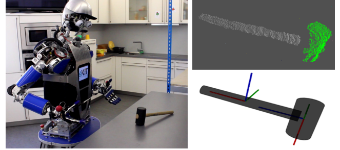
Fig. 8. A grasping task for ARMAR-III and the perceived point cloud together with matched shape primitives.
