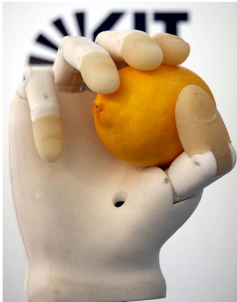
Fig. 1: The KIT prosthetic hand. The underactuation mechanism allows the fingers to adapt to object's shape.
