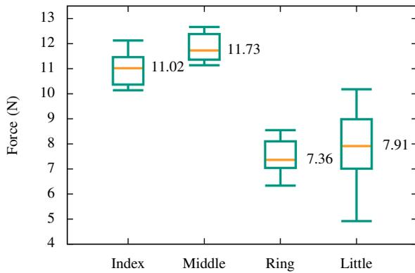
Fig. 7: Triangulated finger tip forces; with the mean value depicted in orange, the upper and lower box boundaries being the first and third quartile and the outer lines denoting the extrema
