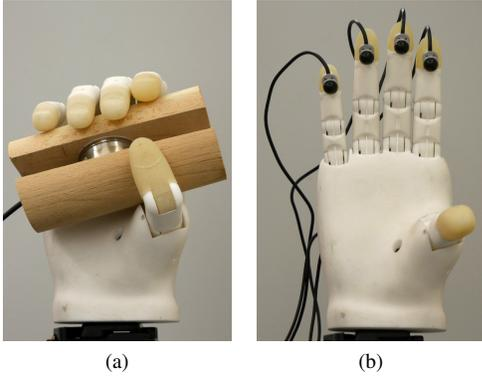
Fig. 6: Experimental setup to measure the power grip force (a) and the maximum finger forces (b)
