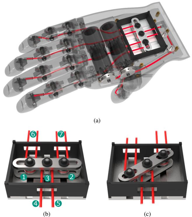
Fig. 2: Tendon routing within the prosthesis (Tendons and guiding tubes in red) (a) and the force distributing mechanism with all tendons pulled equally (b) and with the main rocker rotated caused by blocking the two rightmost fingers (c)
