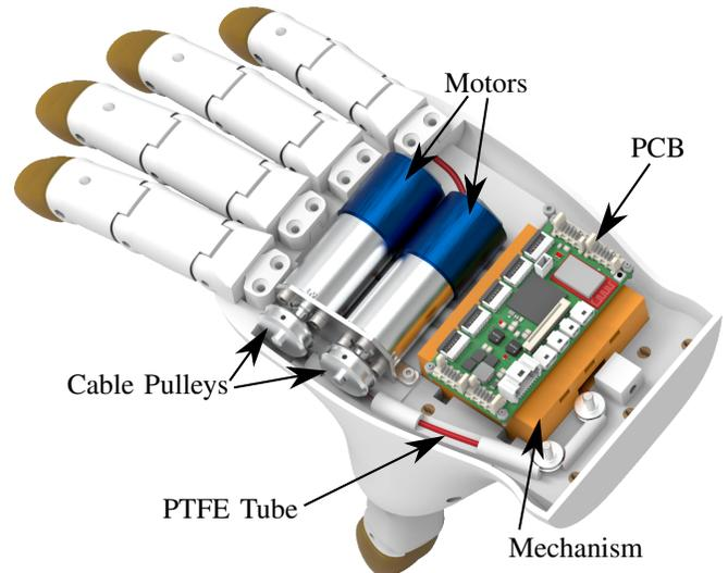
Fig. 3: The components integrated inside the prosthesis palm: motors, embedded system and underactuated mechanism
