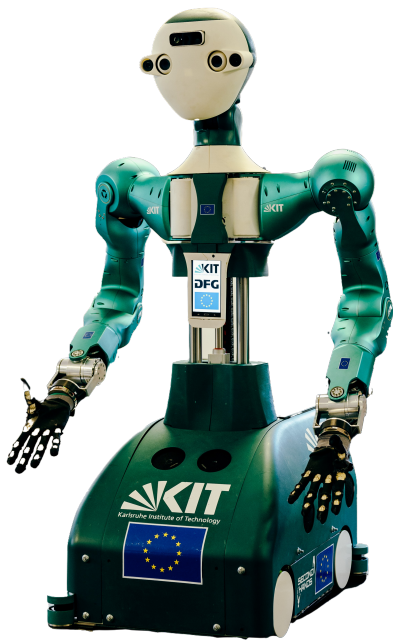
Fig. 2. The humanoid robot ARMAR-6, leveraged for its adjustable torso height and various camera angles provided by its adjustable roll-yaw neck, to enrich our dataset.
